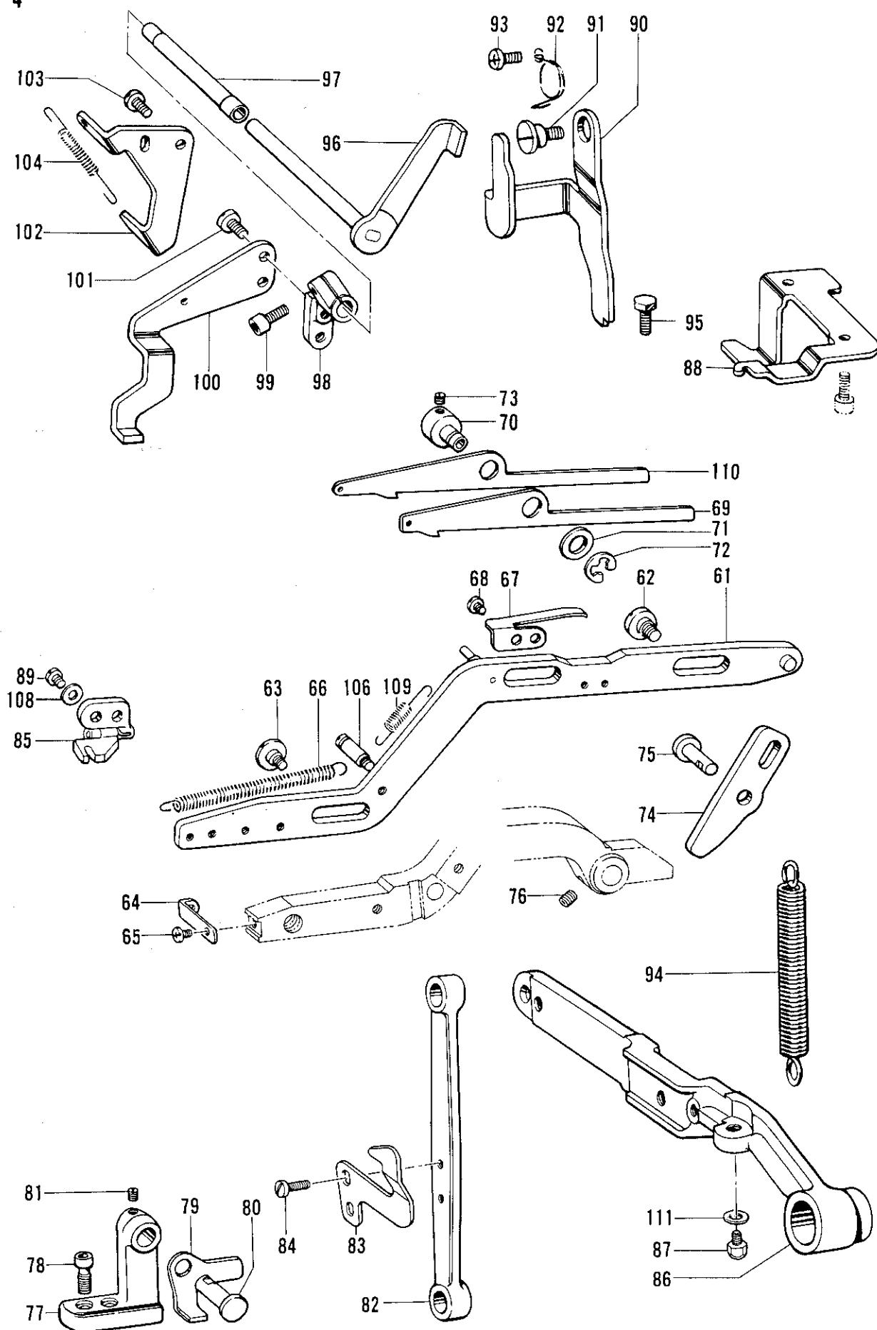
W. 上糸切り関係 (2) /Upper thread trimmer mechanism (2)/Oberer Fadenabschneider (2)/
