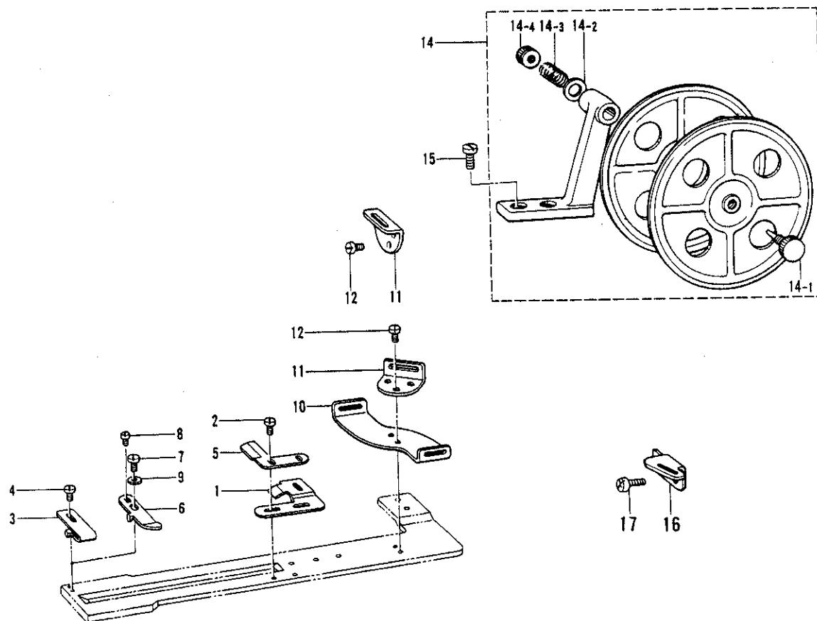
P. 糸切れ感知関係 / Thread breakage detector mechanism / Fadenbruchfühler /
