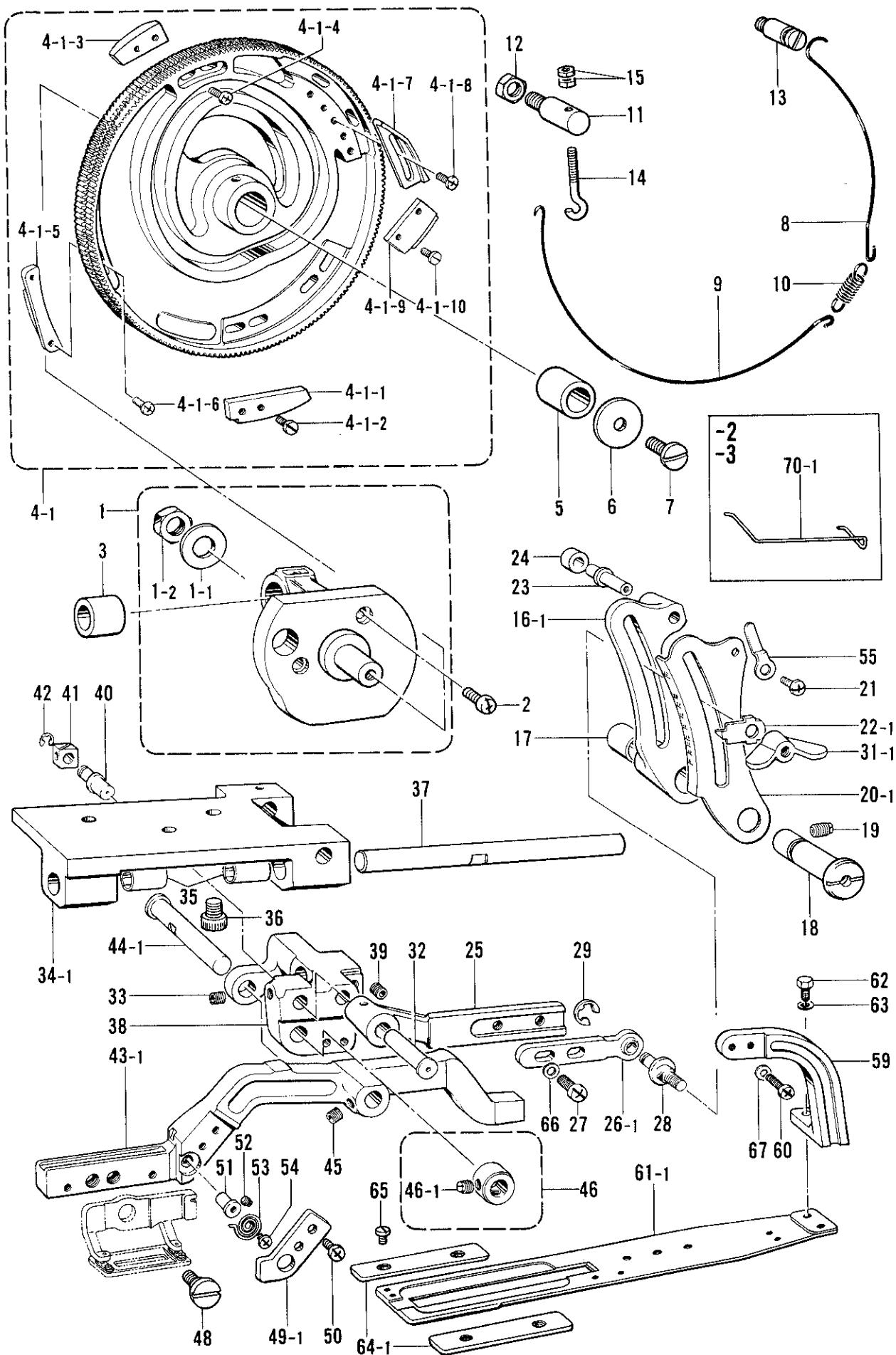
L. 送り関係 (1) /Feed mechanism (1)/Transportvorrichtung (1)/
