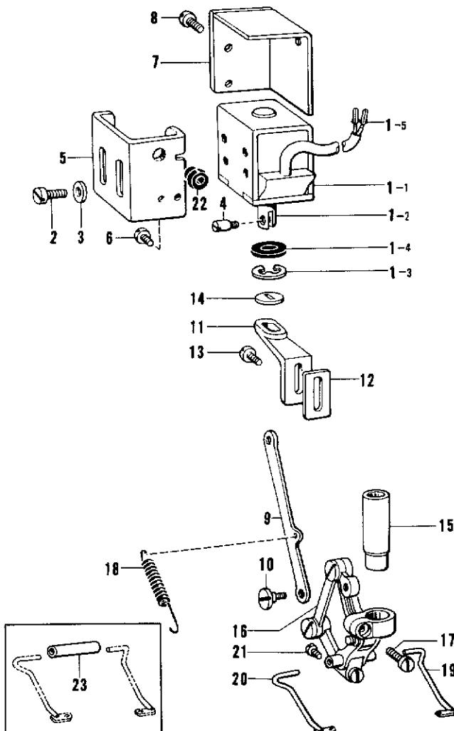
**P. Quick reverse switch mechanism [-400A..-700A..-900A]**
