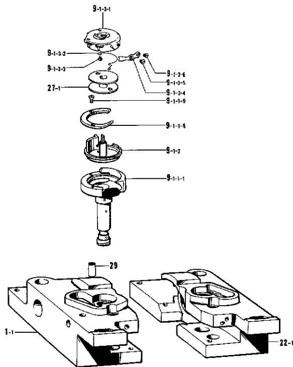
**K. Rotary hook mechanism (3)(-400A--700A--900A)**
